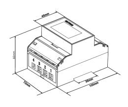
Height 100mm Width 72mm Depth 66mm
